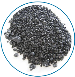
Iron silicate granulate, similar to natural volcanic glass, e.g., obsidian
