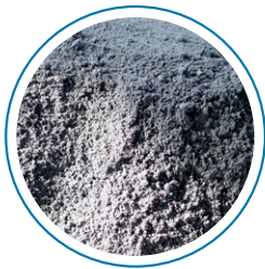
Iron silicate fines, similar to mineral flour
