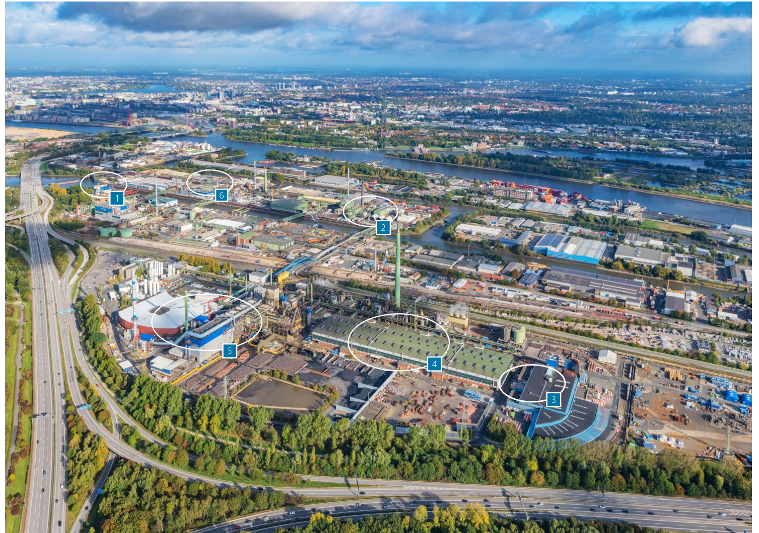
1 Continuous casting plant 2 Secondary smelter/precious metals 3 Rod plant 4 Tankhouse 5 Primary smelter (RWO) 6 Administrative building
