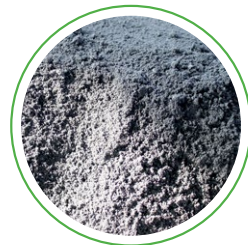
Iron silicate fines, similar to mineral flour
