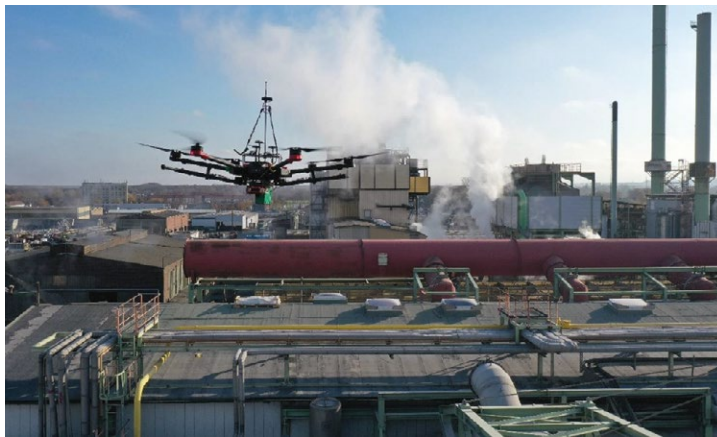
Emission measurements with drones at the Lünen plant
