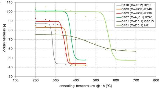
The softening behaviour of various copper alloys with high conductivity is displayed. CuZr0.1 has a very good stability against softening.
