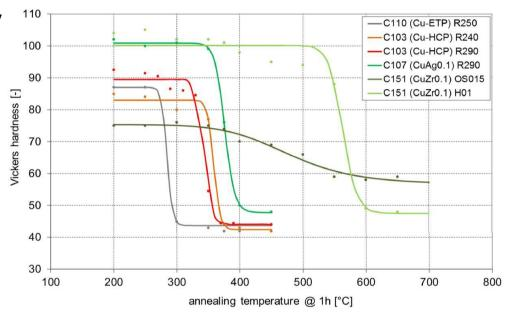
The softening behaviour of various copper alloys with high conductivity is displayed. CuZr0.1 has a very good stability against softening.
